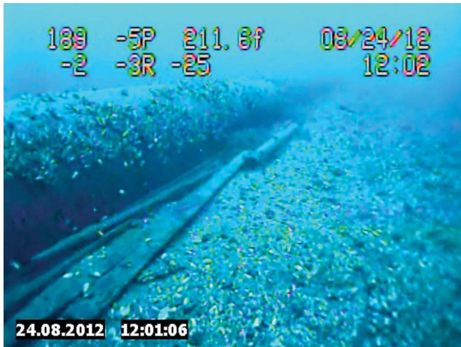
Figure 6. Photo Clipped from Enbridge 2012 Underwater Inspection Video of the West Line Taken on 8/24/2012 at 12:01:06 Showing Detached Slats.
