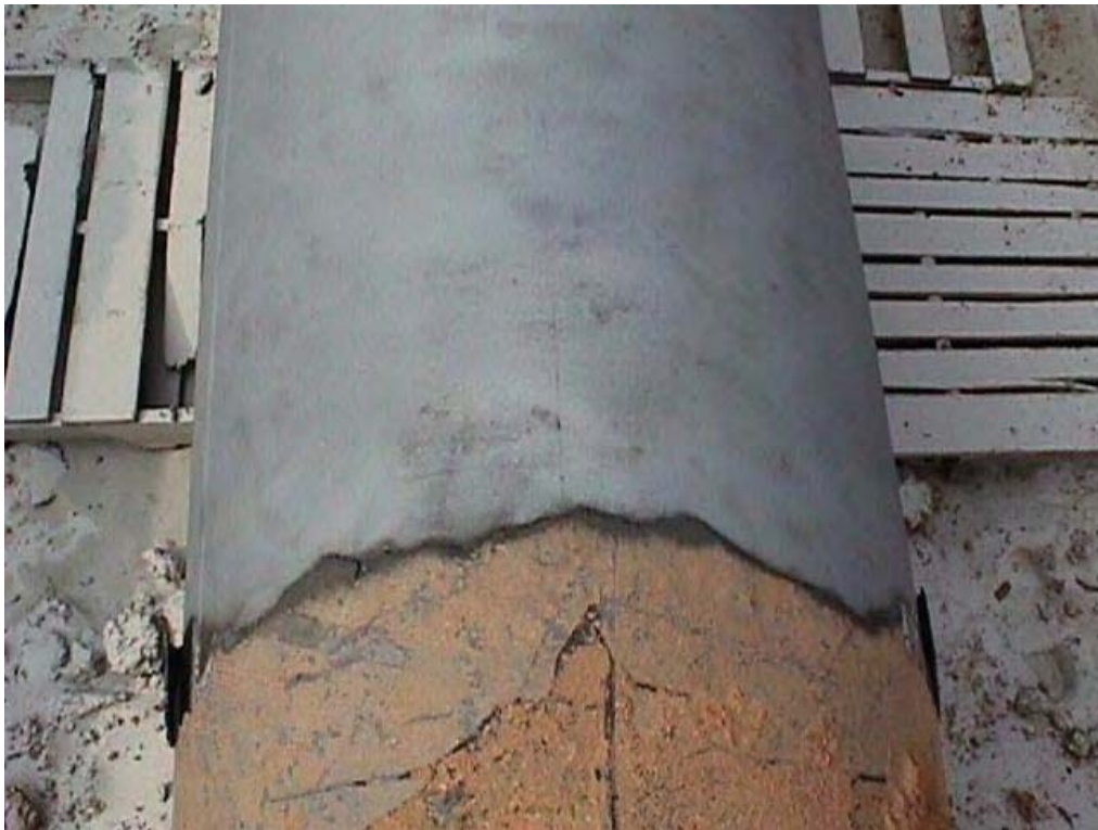
Figure 12. Typical Corrosion Found Under a Disbonded Coating as Reveled by Light Abrasive Blasting
